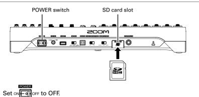
2. Open the SD card slot cover, and insert an SD card all the way into the
