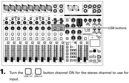
The signal controlled by the channel is switched to the USB audio channel signal (before EQ).
