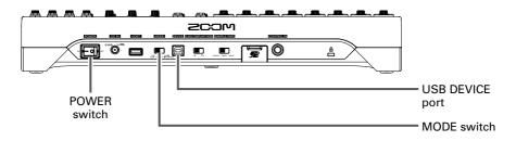
**1.** Use a USB cable to connect the USB DEVICE port to the computer.
