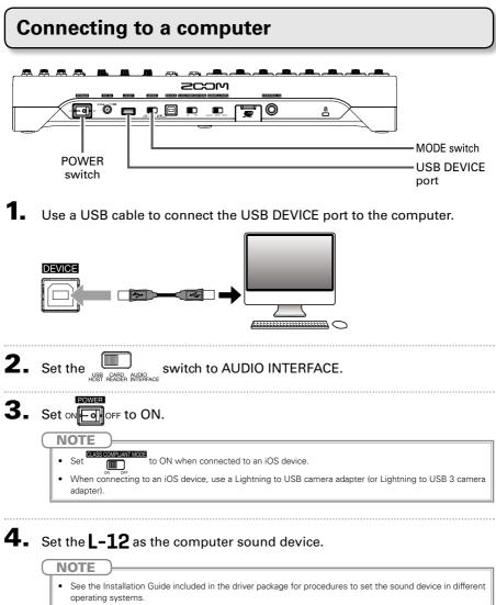
· Audio interface functions cannot be used when the sampling rate is set to 96 kHz.
