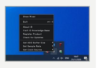
For mixing, buffer size of 256 should be perfect. For tracking, experiment with lower buffer size values. How powerful your computer is, and how processor hungry your project is, will affect how low you can get the buffer size settings before you get audio instability.
