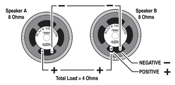
COMBINATION OF SERIES & PARALLEL: This is really just two sets of Series wired speakers connected in Parallel. This is how you maintain a consistent load with multiple speakers. The importance of this is more evident when you have more than one cabinet
