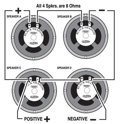
to connect to your amplifier. This is when you need to figure out the loads and how to wire them up without applying too low of a resistance on the amplifier.
