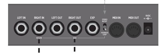
Connect an external effect to the feedback loop. Any external effect can be used. Feel free to experiment with the different sounds that can be achieved. All of the delay repeats will be processed through the external effect.
