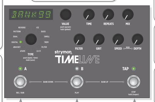
**FOOTSWITCH A:** Press to engage or bypass preset A of the current bank. Hold to activate infinite repeats. **Looper Active:** Activates record if there is
