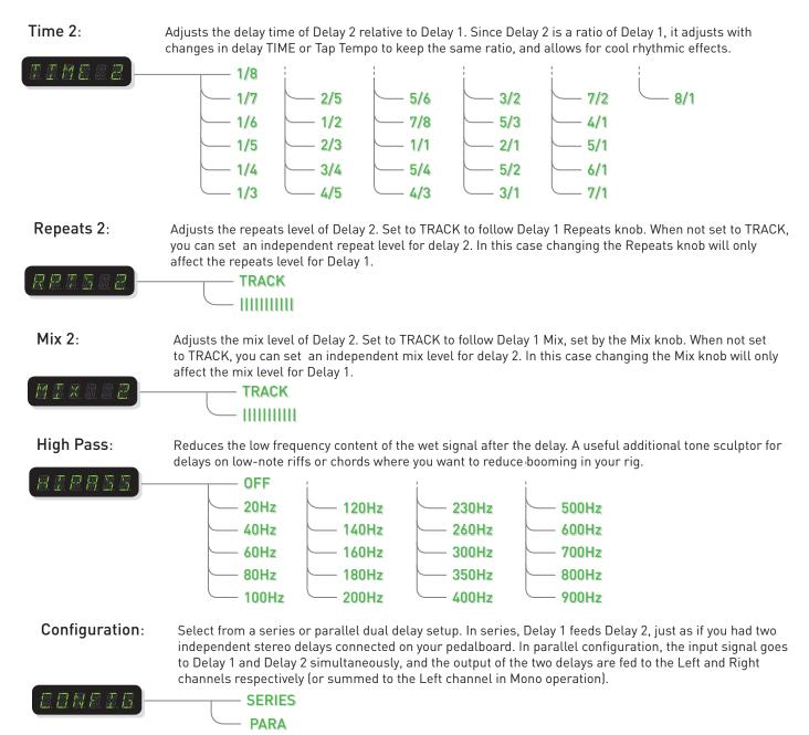
**TIPS & TRICKS:** Set the CONFIG param to PARALLEL to get independent Right and Left channel delay lines (the two parallel delays will be summed to mono in mono operation - very useful for rhythmic delays). This also allows for a 'wet - dry' stereo setup as follows:
