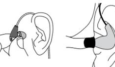
**Important:** If there seems to be a lack of low frequency response (bass), this means that the earphone sleeve is not forming a tight seal. Gently push the earphone deeper into the ear canal or try a different sleeve.
