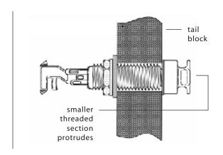
With the jack in place, lay the remaining washer over the threads and attach the external retaining nut until it's tight. Finish by attaching the strap ring (it should cover the retaining nut and washer). Note that asserting too much pressure may crack the finish.
