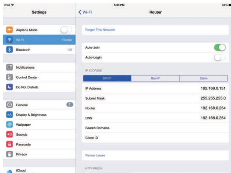
4. Tap [DHCP], and then confirm that the iPad has received settings for IP address, subnet mask, router, and DNS.
