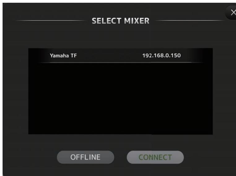
After StageMix has received the necessary data from the console, the mixer window is displayed and you are ready to begin using StageMix.
