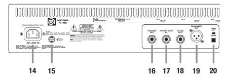
14. AC LINE IN: This is where you connect the supplied AC power cord. Plug the male end of the cord into a grounded AC outlet.
